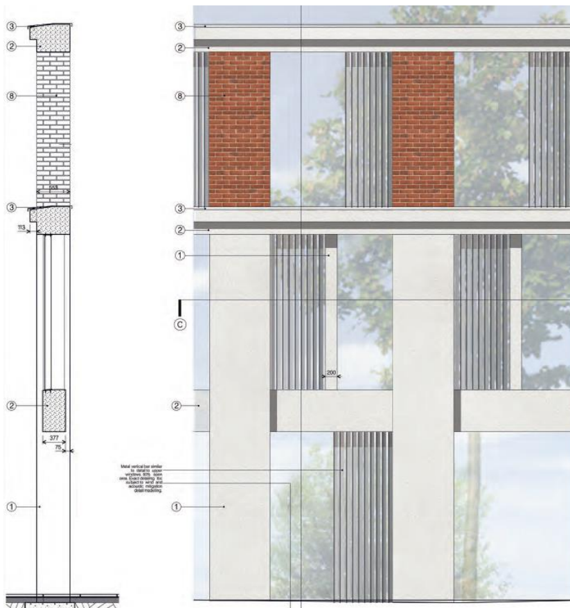
Detailed Elevation of Perimeter Colonnade
